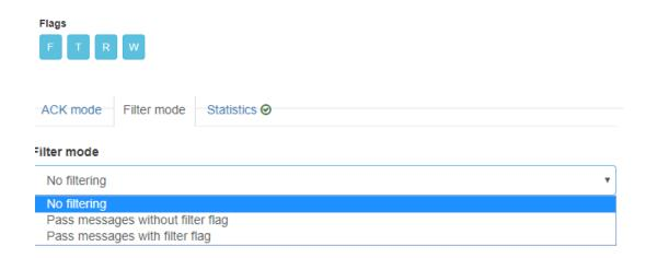
1.4.3. **Statistics** – receive statistic information to group address – source address / RSSI signal level / TX power. Statistics telegram can be sent on all valid telegrams which are received by LoRa.
